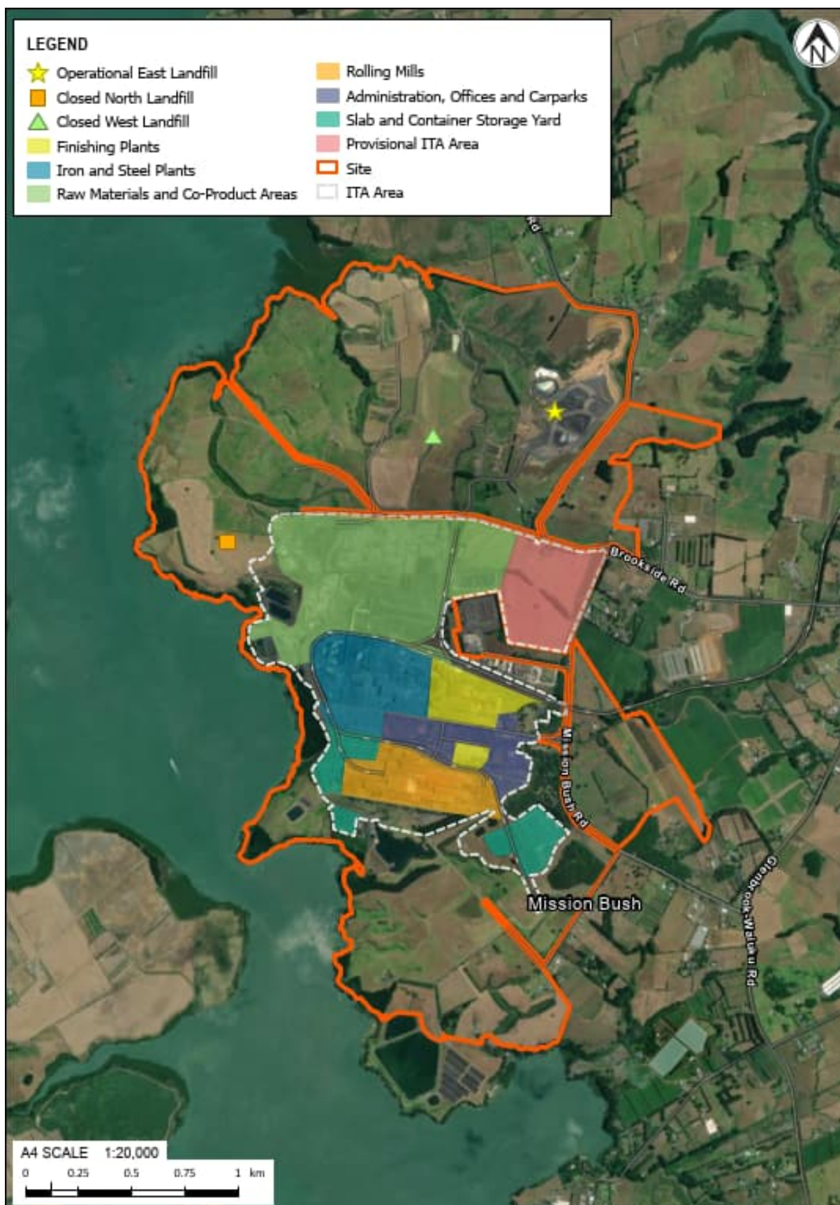
Figure 4.3 Indicative Steel Mill Plant and Process locations (reproduced from Figure W7 of the AEE Report).
